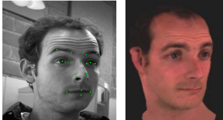
Tracked features are shown as green points in video images (left), producing animations that include deformations and skin wrinkles (right) created by volume morphing and appearance classification.
