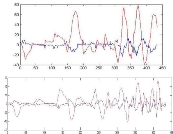
The graphs above show the values of (x's, y's) of the camera trajectory before (in red) and after (in blue) the stabilization process. The blue curve shows much smoother transitions as compared to the red one, clearly indicating the ongoing stabilization process
