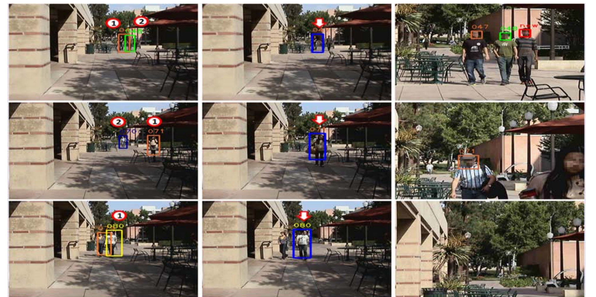
(a) Person detection and tracking (b) Select a person to Zoom in (c) Face detection and association
