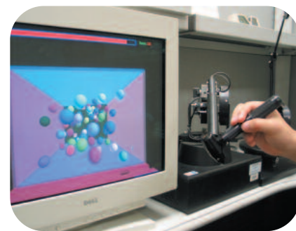
A researcher holds a robotic force-feed device, called a PHANToM, and moves a ball around in a virtual environment. He will feel resistance if his ball bumps into other balls.
