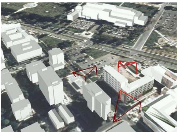
An Augmented Virtual Environment (AVE) image showing three video projections as red wire-frames around a USC campus building complex.
